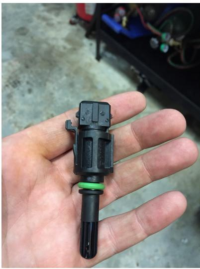
Step 5: Use supplied plug to cover hole where IAT sensor plugs into airbox to avoid debris getting in. Bending of the tabs on plug may be required to stay tight.
