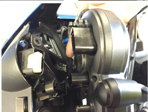
Step 8: Drill hole directly to the left of the hump for mounting of IAT. Gradually step sizes from 1/8th to final of 1/2". Use the left hole pictured (we tried different placement).
