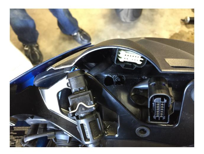
Step 9: Remove clutch side fasteners (5) as pictured with T25 Torx and push fairing forward gently so you have room to run IAT harness.
